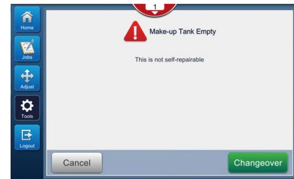
Figure 6: Make-up Tank Empty Fault (E15062)
